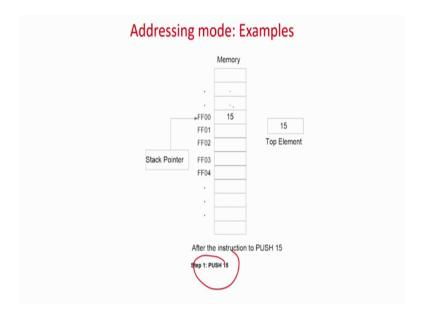
Then we say that push 15; so 15 will be pushed in the top position because it's an infinite stack because this may be available to program one.
