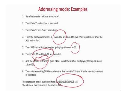
Only 3 steps push, pop, and operate. Push means some elements will be pushed, pop means the top elements will be popped out to the memory buffer and operation means you will operate the top two elements.
