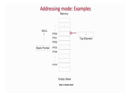
So, this is an empty stack and then this is the stack pointer maybe say that we will start pointing from here this is the top element, this is the whole stack available. And we will do some of the instruction which we have seen in the this question that we will first push 15; then push 12; then 15 then we will add and so on. So, this is the first scenario.
