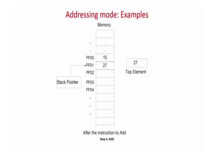
So, it is 15 + 12 is 27. So, 27 is pushed back over there and this is the stack pointer.
